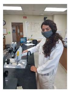
Figure 1: Victoria Konieczka measuring trace element concentrations in sliced spodumene with a Tracer 5i p-XRF unit. Photo by Dr. Larry Lemke, 2020.
