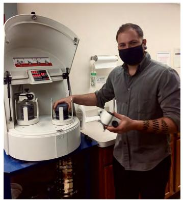
**Photo 1:** Joel Harris preparing a pellet of production sand and cellulose binder to be examined in the high-end WDXRF spectrometer for chemical analysis. Photo credit: Andrew Whaley, US Silica lab technician
