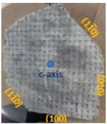
Figure 3: Spodumene from Plumbago North, Maine, cut perpendicular to the c-axis. The Miller crystallographic indices are shown in yellow. The 5 mm x 5 mm grid of >360 points was used for portable XRF analysis.
